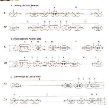
$C - Common \ Link \ \square \ EL - Enlarged \ Link \ \square \ E_{\neq} End \ Link \ \square \ D - 'D' \ Type \ Joining \ Shackle \ \square \ A - 'D' \ Type \ Anchor \ Joining \ Shackle \ \square \ K - Kenter \ Joining \ Shackle \ \square \ S - Swivel \ Piece$
